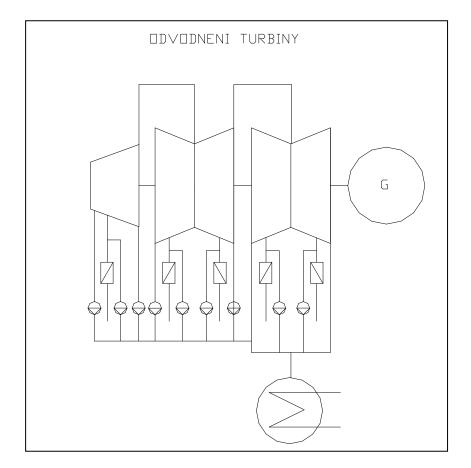
In comparison with the orifice plate system this kind of dehydration is at the beginning nearly lossless, but after one-year-operating, without changing of valves, the loss will get over an amount of 100 000 USD per year.
